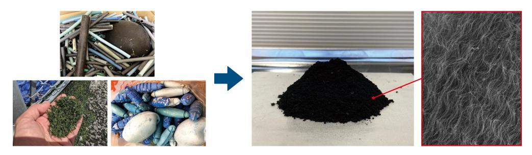
Converting plastic materials such as oyster pipes, artificial turf, and fishing nets into CNTs.
