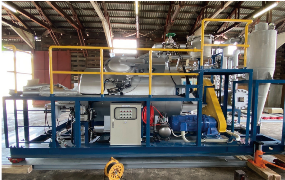
Small subcritical water treatment unit (left) and coal substitute fuel that can be produced from the treated product (right)
